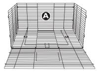
Snap the wire hook through the wire loop.
